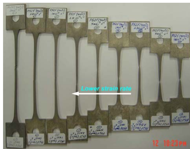
Fig. 2 Deformed samples under various strain rates at 400 °C
